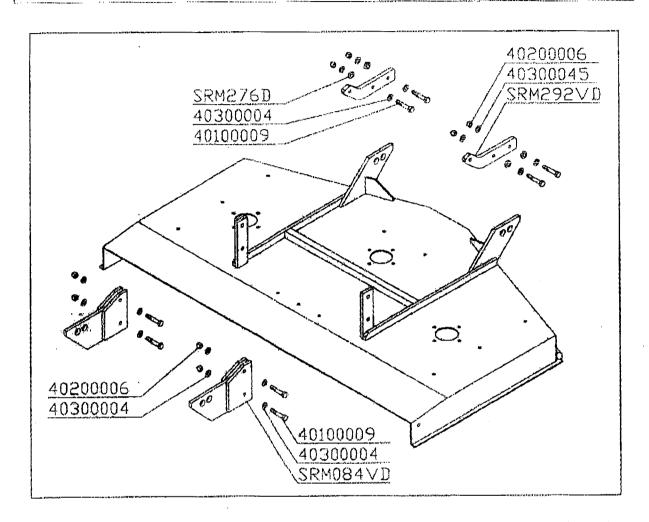
The kit is suitable to transform the rear mowers, rear discharge (PRM) and side discharge (SRM), into front mowers, rear discharge (FMRD) and side discharge (FM). The kit is the same for the three dimensions 120, 150 e 180.
